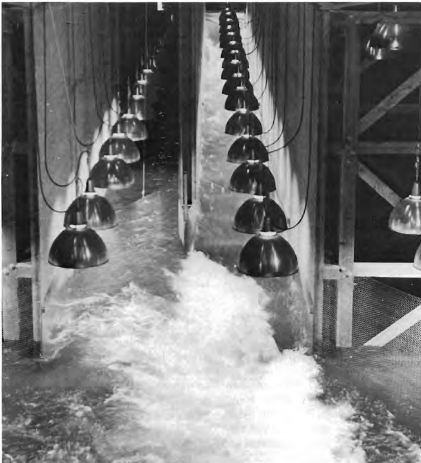
Figure 7.—Experimental channel with a water velocity of 16 feet per second appears on right. Entrance to channel on left is screened to prevent access during swimming ability tests.
