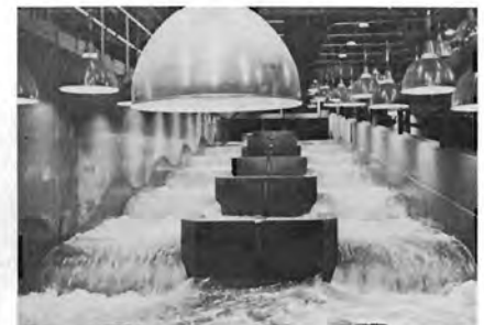
Figure 9.—Test of a full-scale model of a new fishway design in the laboratory.
