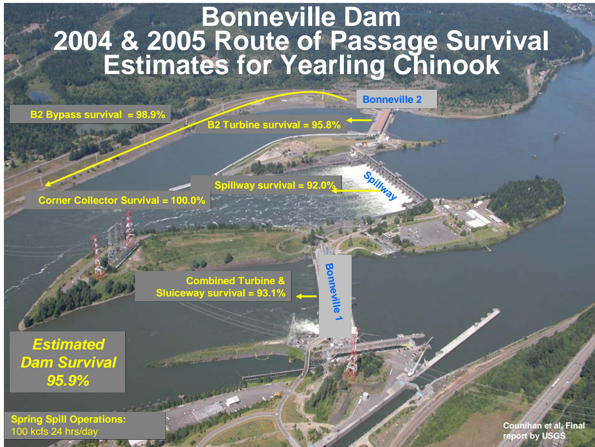
Figure A-6. Route specific dam survival estimates for yearling Chinook for 2004 and 2005.
