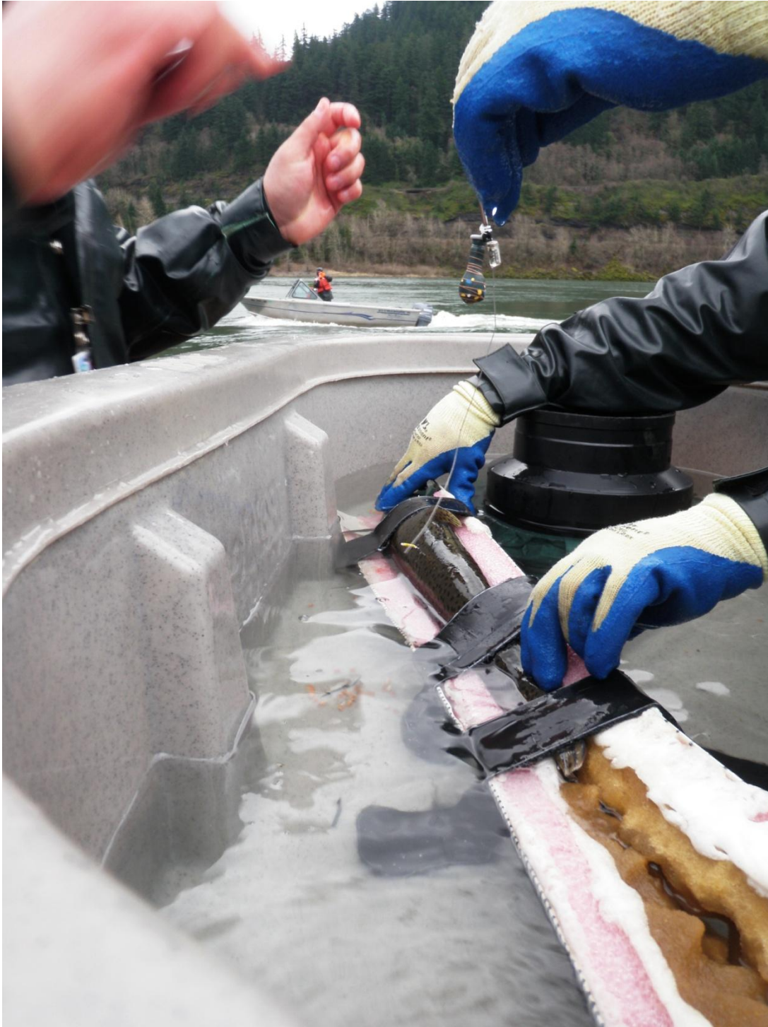
Figure 2-4 Fish restraint device for attachment of HI-Z tags.
