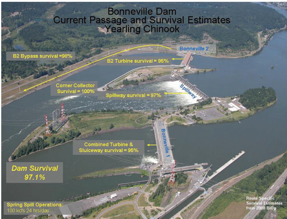
Bonneville Dam — Route-Specific Passage and Survival Estimates for Yearling Chinook Salmon When Spring Spillage Operations Are 100 kcfs All Day
